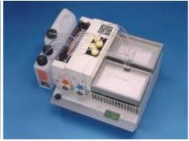
The BioLane HTI robot consists of two systems, a blue and a red system. Each system has 9 plastic tubes hooked into the robot labeled 1 to 9. The robot has been programmed so each tube has been assigned to a specific solution. By inserting the tube into the solution the robot will automatically take the required amount as generated by a script. The robot will gently rock the samples in a tray while the program is in progress.
